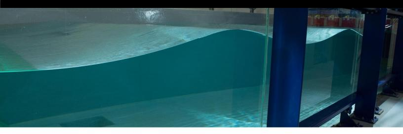
MTU Wave is the collaborative wave tank lab at Michigan Technological University dedicated to advancing research and development in the field of floating offshore technologies. Our wave tank provides highly controlled conditions that enable us to validate complex mathematical models, execute wave energy converter control studies and test the performance of floating or underwater structures.
